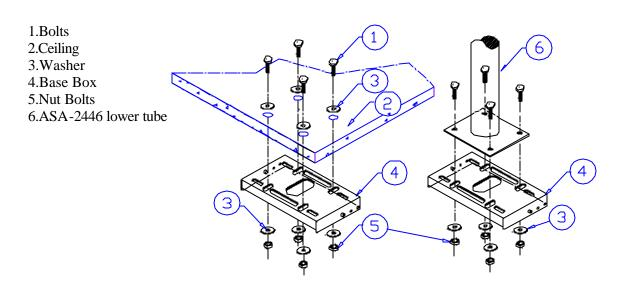
**NOTE:** If **ASA-2446** adjustable height suspension adapter is a part of the installation, securely install the adapter to the ceiling at this time (**see detail above**)
